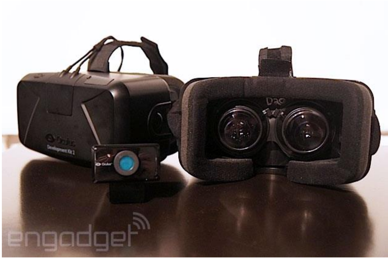
Figure 7. A prerelease version of The Oculus Rift virtual reality headset (Oculus Rift Development Kit 1, 2014).
