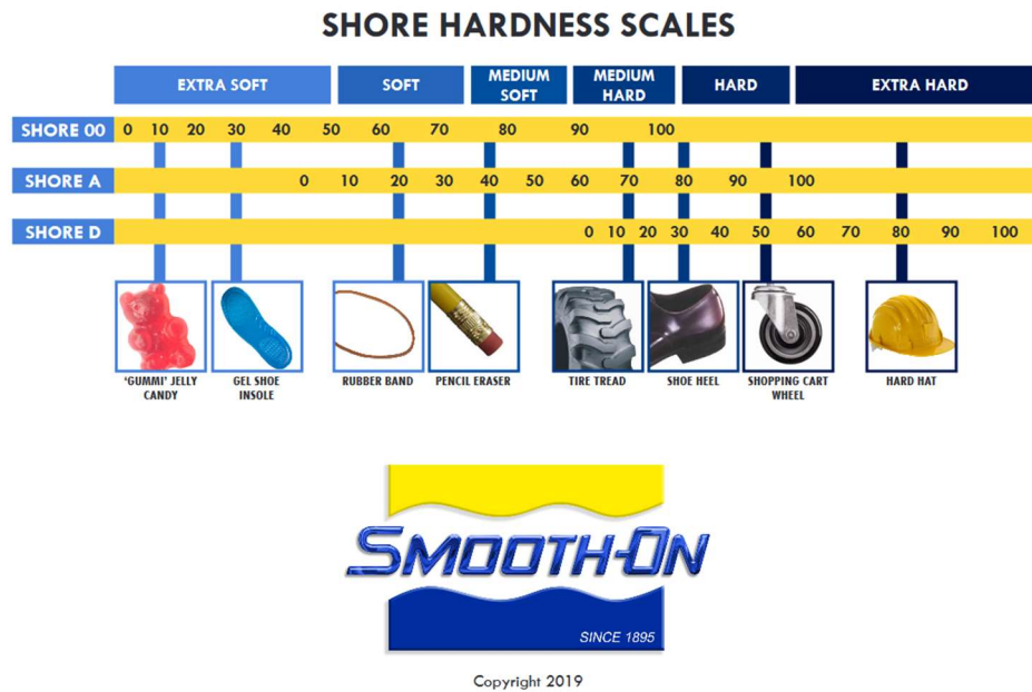
Figure 62: Shore Hardness Scale Material Comparison (Durometer shore hardness scale, 2019)
