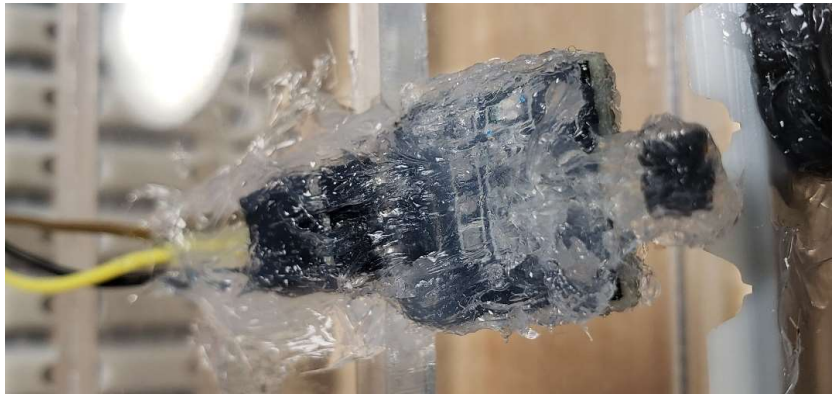
Figure 74: Hall effect Sensor Covered in Silicone Sealant
