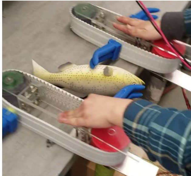
Figure 92: Intake mechanism working to intake a rubber fish to showcase to demonstrate functionality
