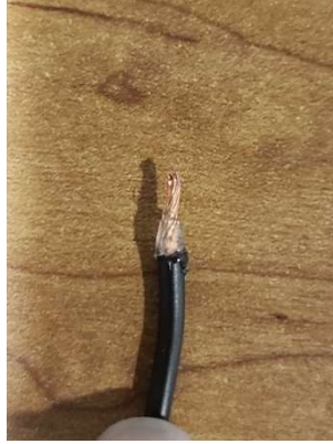
Figure 43: Saltwater Basin Measurement Probe Silicon Encased Wire
