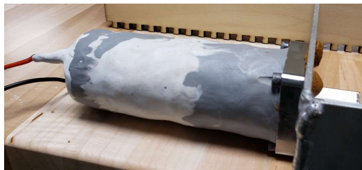
Figure 73: AndyMark PG 71 Motor Encapsulated in Sugru
