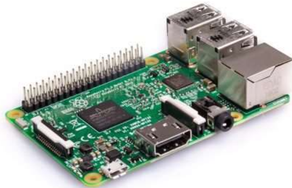
Figure 16: Raspberry Pi3 Model B (Raspberry Pi, 2018)
