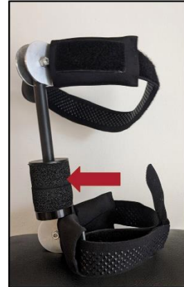
Figure 25. NBR component of brace prototype
