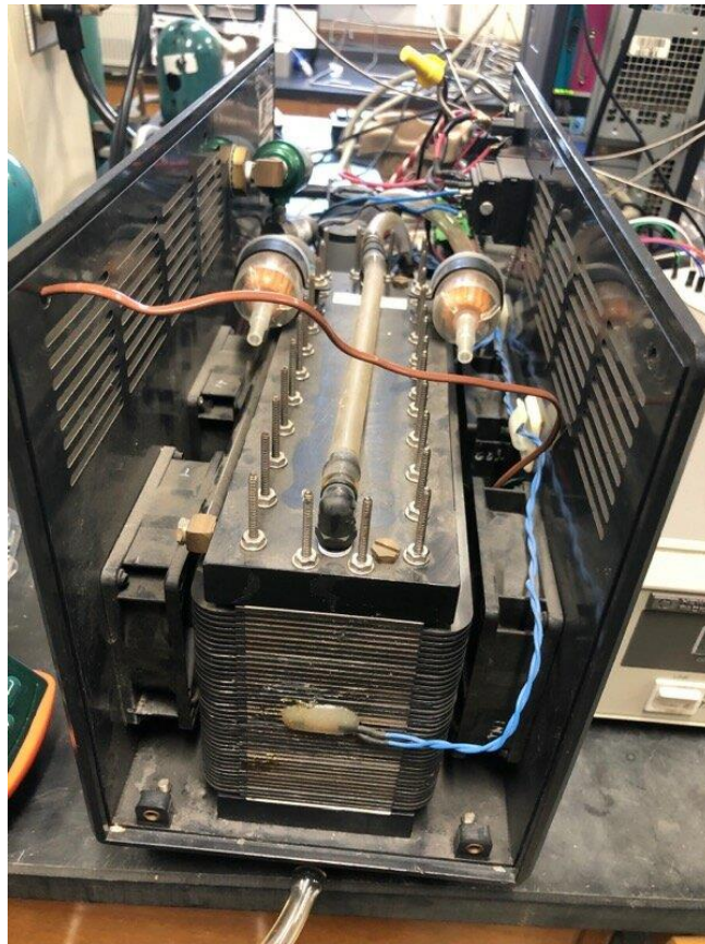
Figure 19: Front view of the PowerPEM-PS250 fuel cell used for experimentation
