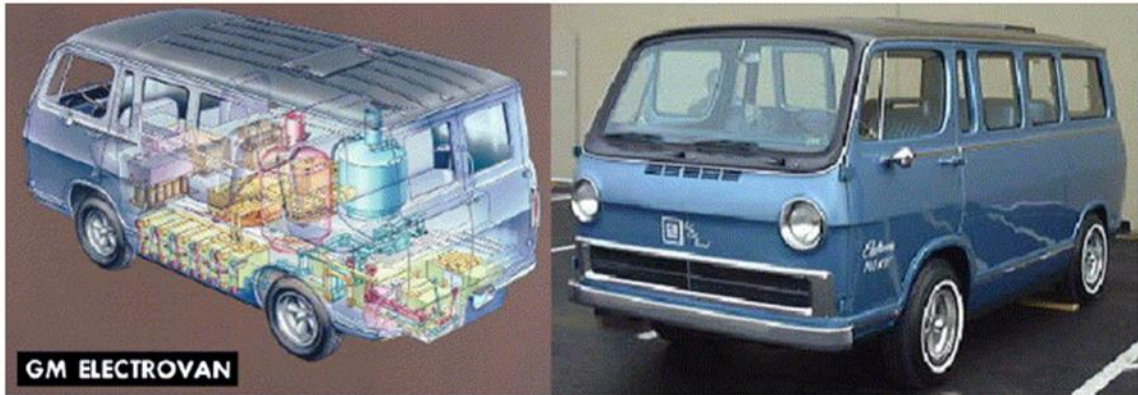
Figure 6: 1966 General Motors Electrovan, which shows the fuel cell system with all of its components (Helmolt and Eberle, 2007)
