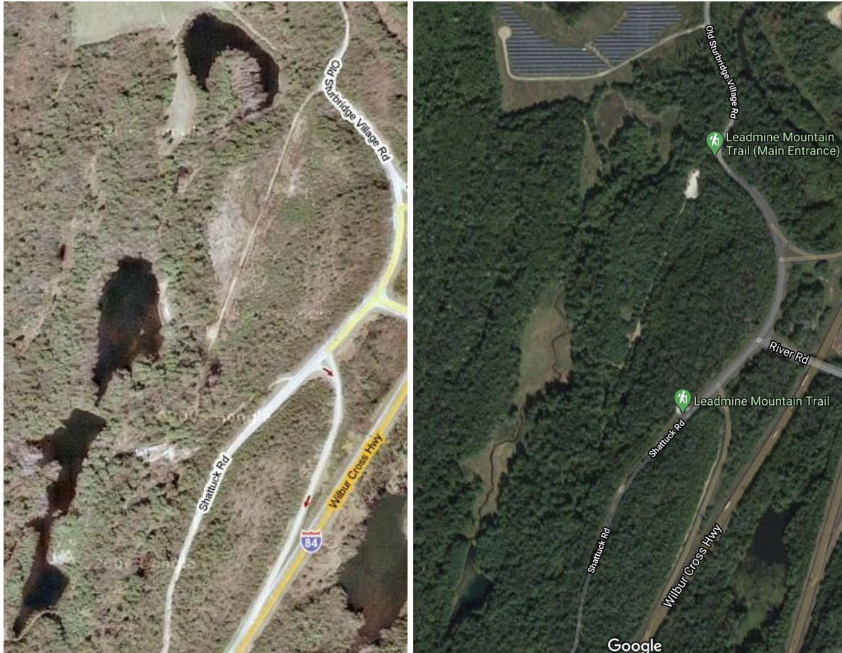
Figure 4.1.2 - Hamant Brook Changes - Pictured above are aerial views of the Hamant Brook before and after the removal of the dams in 2017, taken in 2007 (left) and 2020 (right), respectively. The swimming and boating lakes seen in figures 3.1.6 and 3.1.7 can be identified in the left photo, whereas the recent, post dam removal photo shows the brook back to its natural course (Camp Robinson Crusoe, 2014; Google Maps, 2020).
