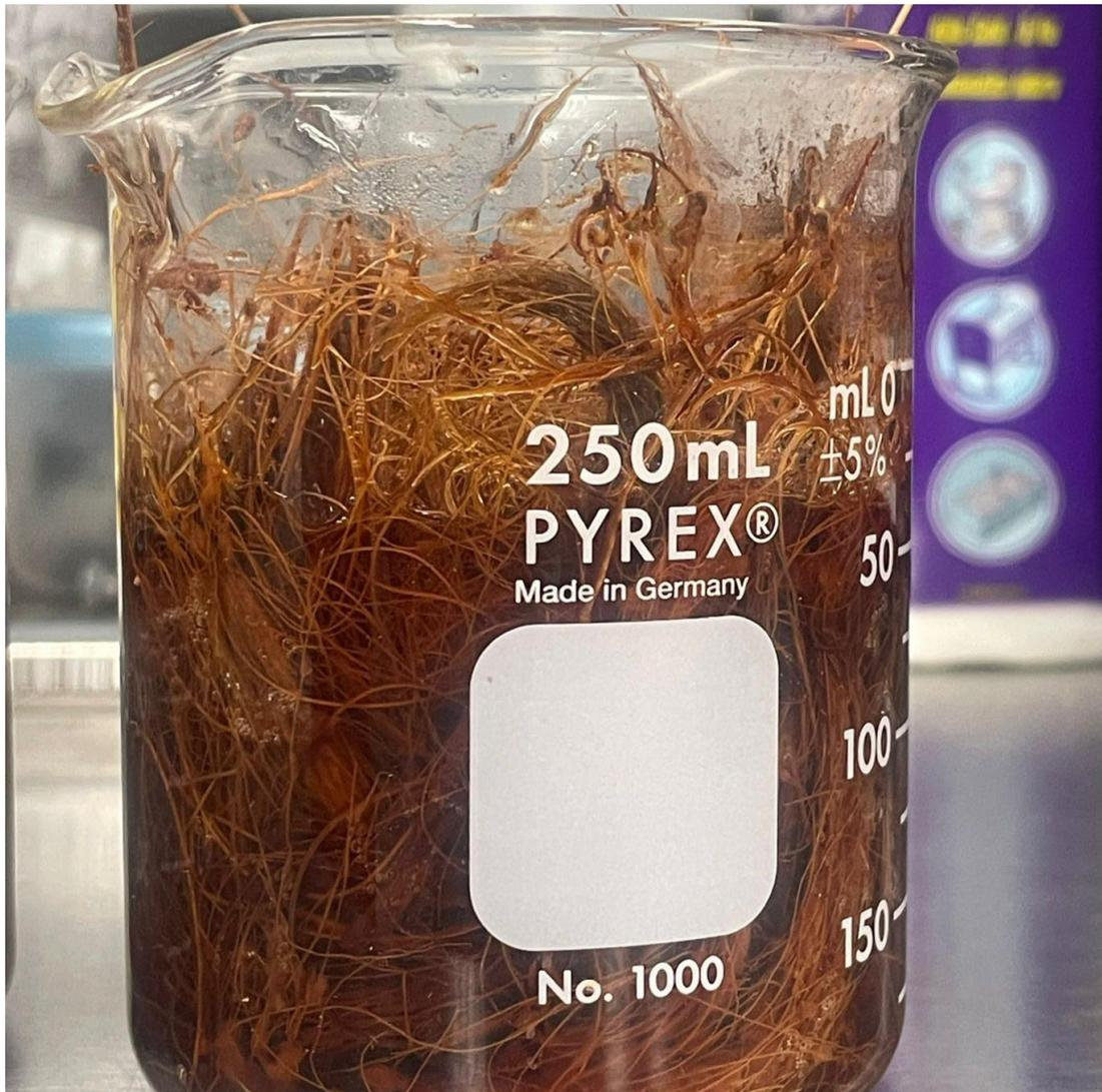
Figure 3.4. Coir treatment in distilled water.
