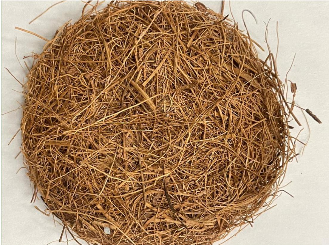
Figure 3.6. Compressed randomly oriented coir.
