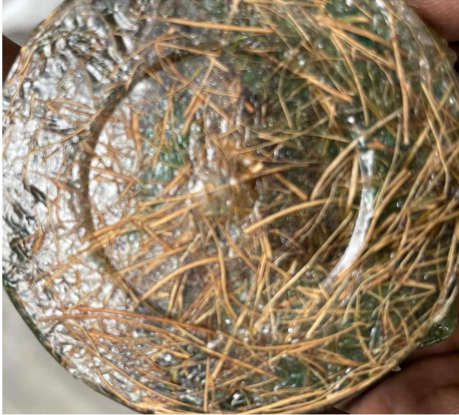
Figure 3.8. Coir Reinforced rPET composite.
