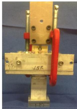
Figure 5.4: Prepared specimen for cyclic and tensile testing.
