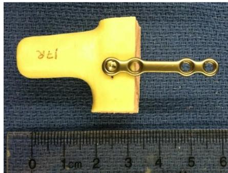
Place the sample between the guide rails for the potting fixture so that the median cut is level with the top of the guide rails, the plate is centered, and the plate remains vertical.
