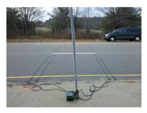
FIGURE 9. INSTALLED TUBES ON ROUTE 140 SB
