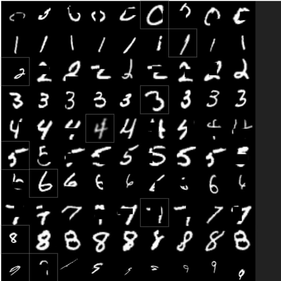
FIGURE 2.15: Examples of multiple series from the random anomaly detection data set with sequence length set to nine. Each series is presented horizontally with the anomaly outlined by a light grey square.
