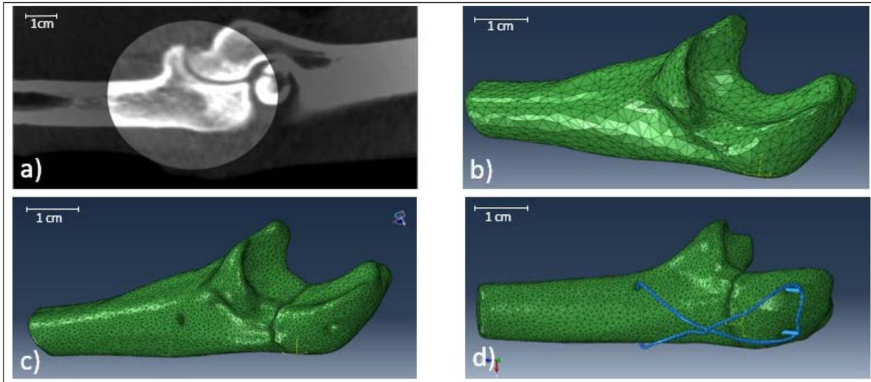
**Figure 3: Development of the model: a) CT scan image of a normal elbow joint b) Normal ulna model from CT scans in Abaqus c) Fractured ulna with holes for TBW hardware d) Ulna model with TBW hardware**
