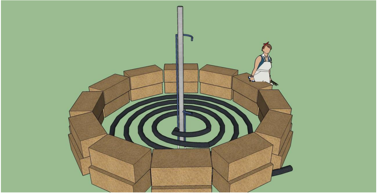
Figure 2: First two layers of hay bales placed around 12 foot diameter base, with aeration tubing extending through insulation
