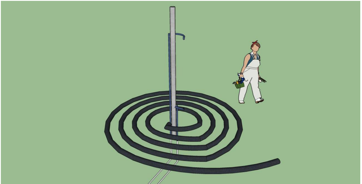
Figure 1: Aeration tubing (black) is laid in concentric circles around the center stake
