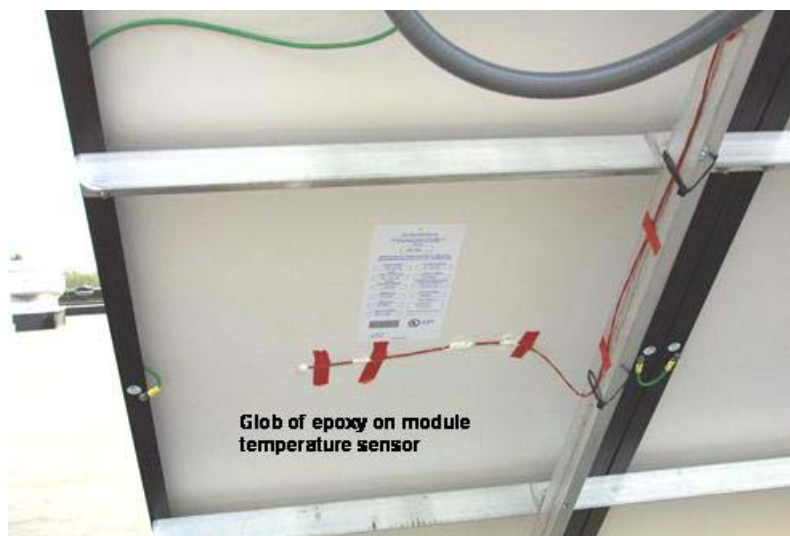
Figure 4. Photograph showing attachment of the module temperature sensor to the back of the photovoltaic module.
