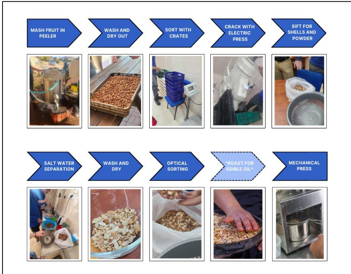
Figure 2: The argan oil-making process at Kibbutz Ketura. This figure demonstrates the stages of argan oil production that lead to oil separation. The roasting for the edible oil stage is optional.
