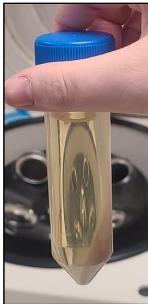
Figure 8: 45 mL sample of oil spun at 5750 RPM for one hour. This figure demonstrates how a sample should look at opacity level 5. The solids are visible at the bottom right of the container.
