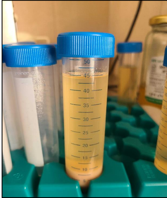
Figure 4: Gravitational settling method in progress. 45mL of oil was used to find the gravitational separation rate for 14 days. The yellow liquid is cloudy oil and the white paste at the bottom is the separated sediment.
