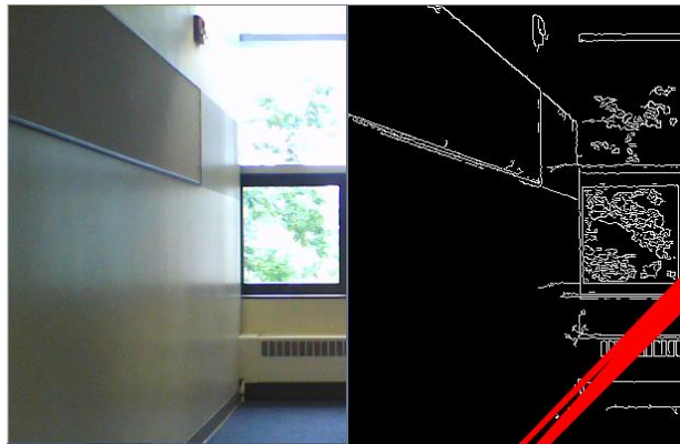
Figure 27: Inclined floor edge detection
