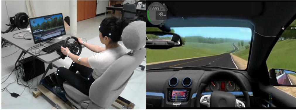
Figure 6.4: A participant is driving in fixed-base simulation testbed within motion capture laboratory. (Left): Experimental setup. (Right): Screen capture of the driving simulator game.
