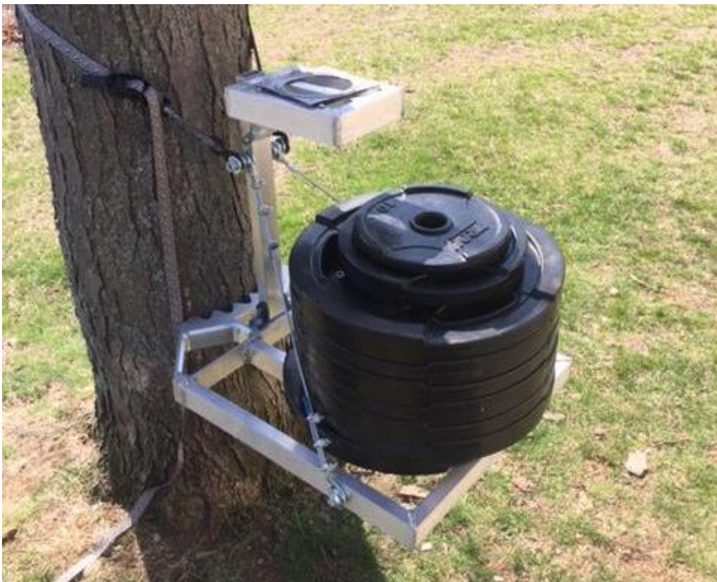
Figure 17: Tree Stand supporting 350 lbs.
