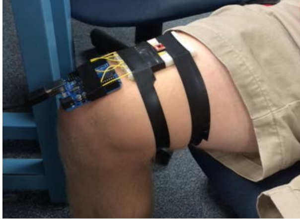
Figure 27 - Accelerometer Testing Setup
