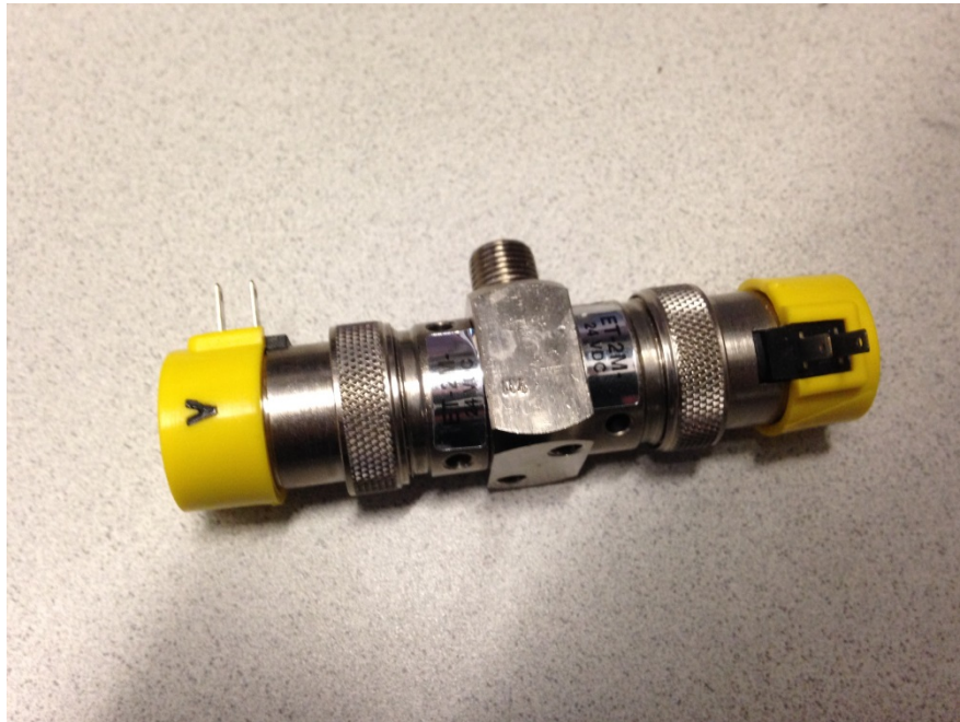
Figure 55 - Clippard 2-way Manifold Mount Solenoid Valve Model ET-2M-24
