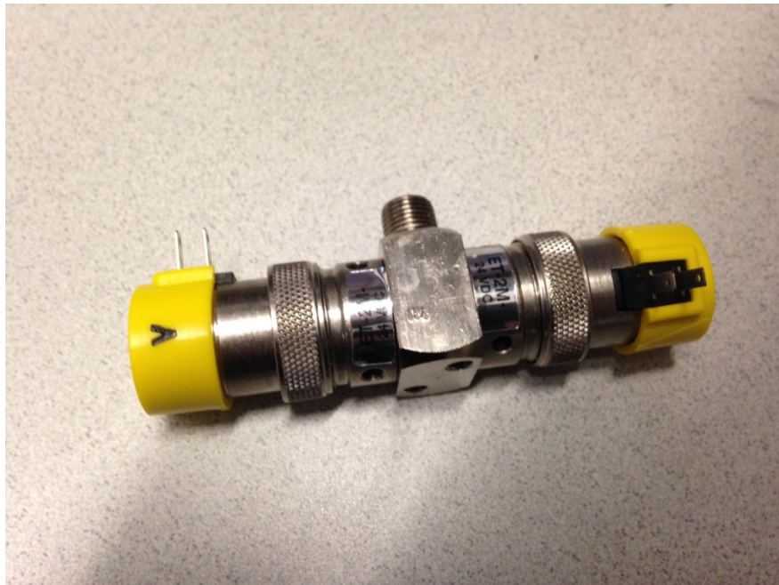
Figure 20 - Clippard 2-way Manifold Mount Solenoid Valve Model ET-2M-24
