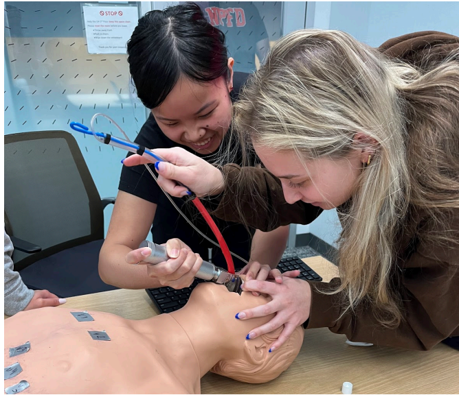
Fig. 75. This image shows the device being placed into the intubation mannequin, with the help of a laryngoscope to guide it. The device was easily able to be inserted and removed without damage.
