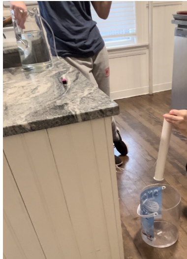
Fig. 21. Initial proof of concept testing. A siphon system was set up to run water through a small tube, representing a ruptured esophageal varix. The large white tube represents the esophageal wall. A balloon was inflated in the white to show cessation of water out of the bottom of the tube, representing cessation of bleeding.
