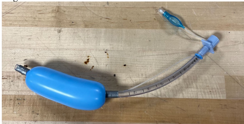
Fig. 42. Inflated balloon on the human endotracheal tube. This model used previously-installed aspects of the endotracheal tube, such as the built-in inflation line to show proof-of-concept for the inflation of a larger and longer balloon on a similar size medical tubing.
