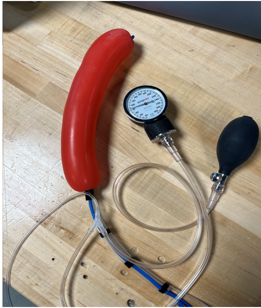
Fig. 70. The device is able to inflate to a particular pressure and can maintain that pressure for an extended period of time. This image shows the device with the balloon inflated by the inflation bulb, holding air, and the bulb and pressure gauge are also visible.
