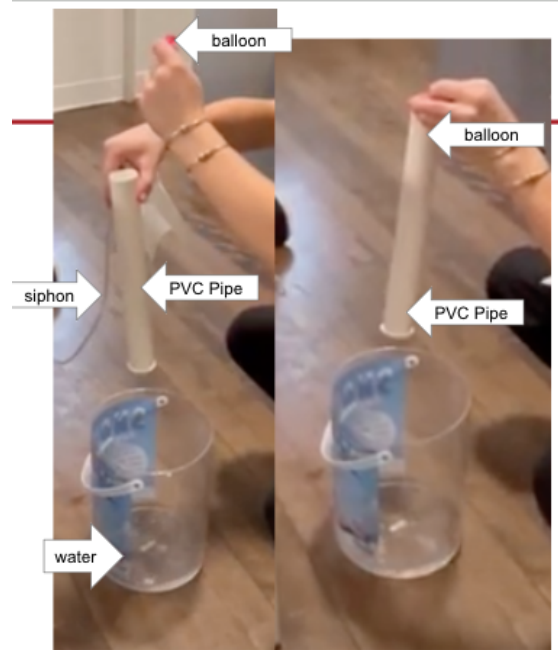
Fig. 47. This figure depicts the flow of water with and without the balloon inflated in the PVC pipe. The left image shows motion in the water at the bottom of the bucket, as the water is running through the PVC pipe and into the bucket because nothing is in the tube preventing it. The balloon is still in the team member's hand in the left image. The right image shows no flow through the tube, as the balloon is inflated in the top of the PVC pipe and thus preventing the flow of water through the pipe.
