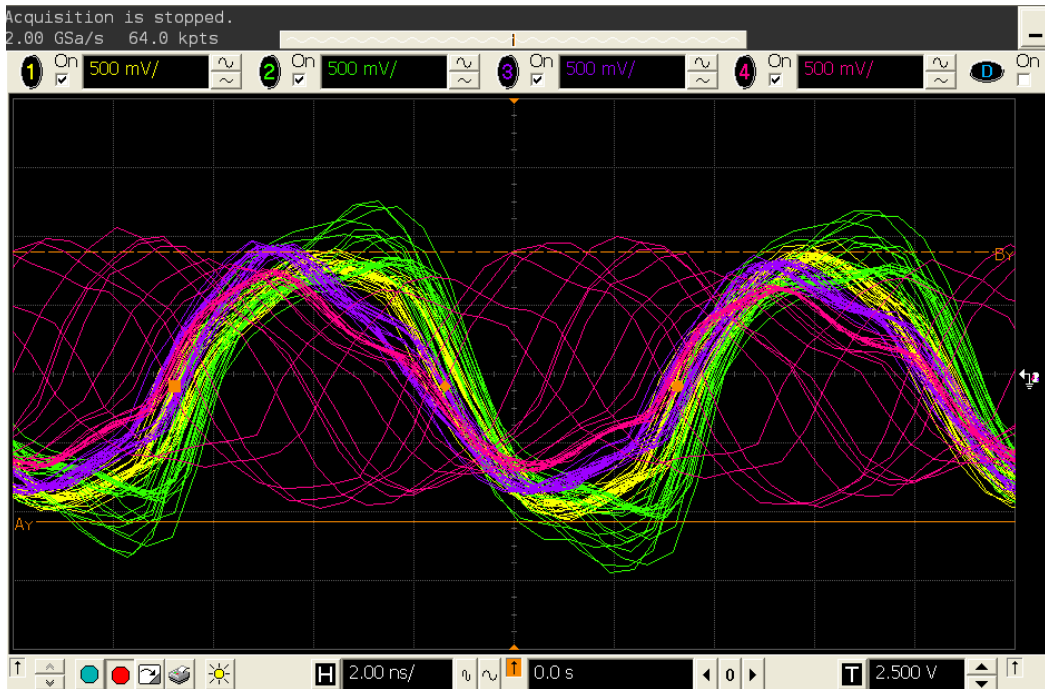
Figure 44: Example with only three of four radios synchronized. In this example, Radios connected to channels 1, 2, and 3 had a reference clock input; the radio connected to channel 4 did not. The x-axis shows time with 2 ns/division and the y-axis shows the signal voltage with 500 mV/division.
