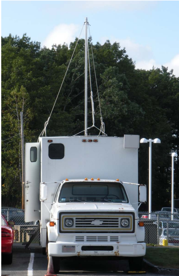
Figure 63: Group 33's mobile transmit station. The BAE transmitter and antenna are the same used in the previous test.
