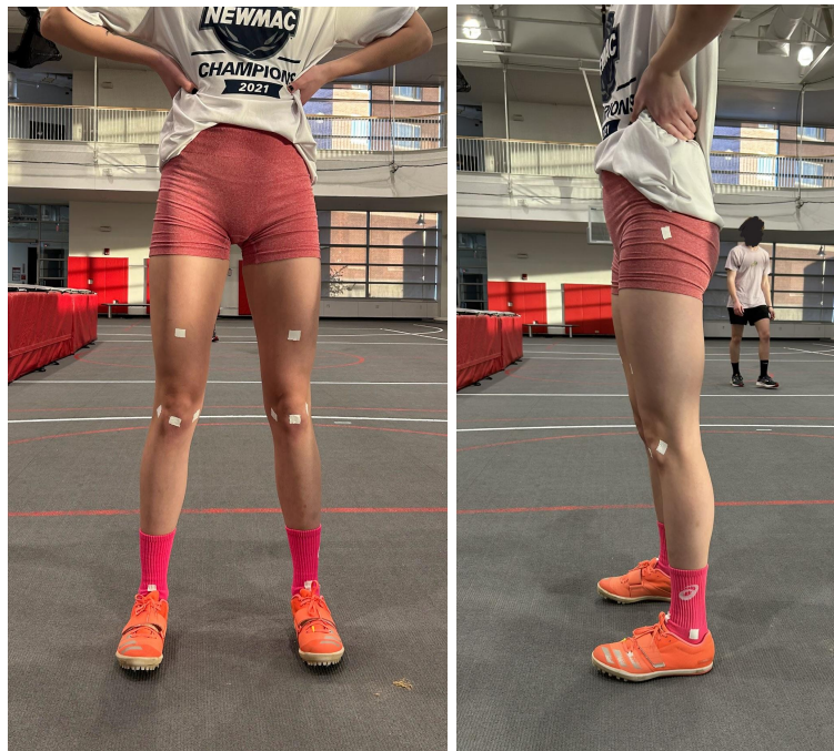
Fig. 5.5 Frontal (left image) and sagittal (right image) view of marker placement with athletic tape.
