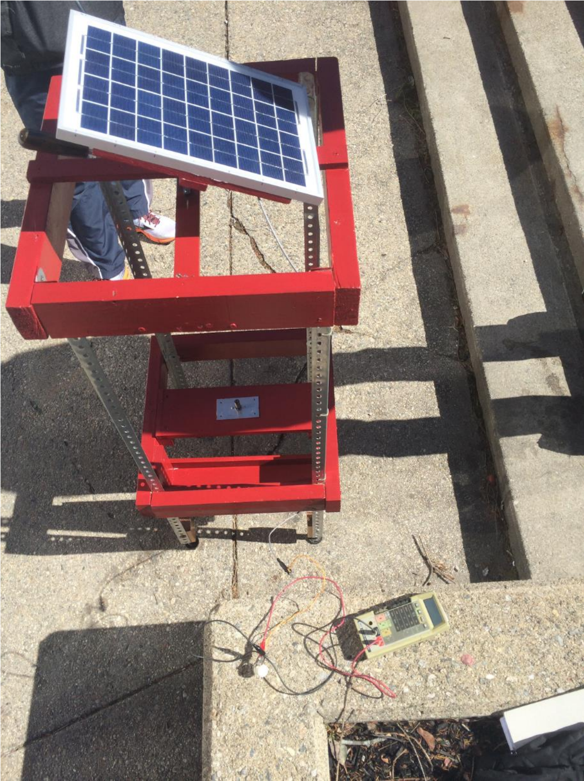
Figure 4-8: Outdoor Environment for Testing the PV Module
