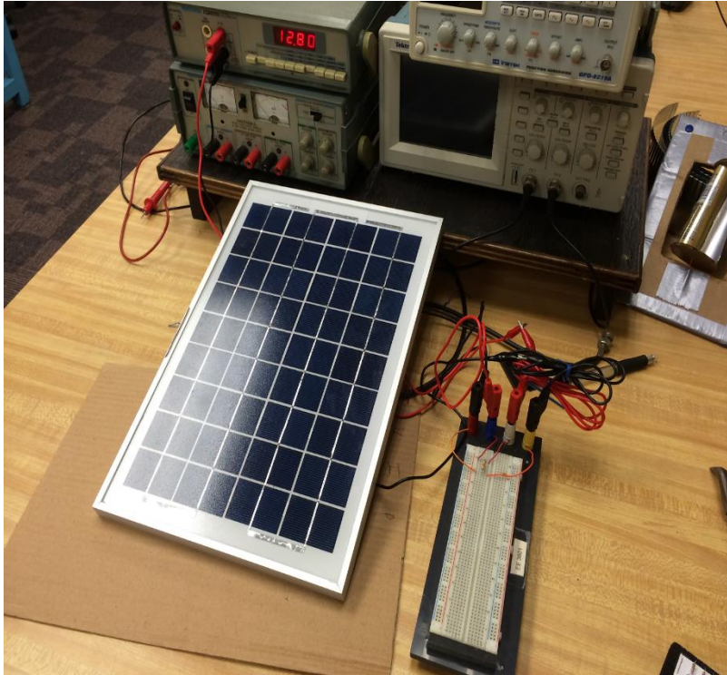
Figure 4-1: Indoor Test Environment for the PV Module
