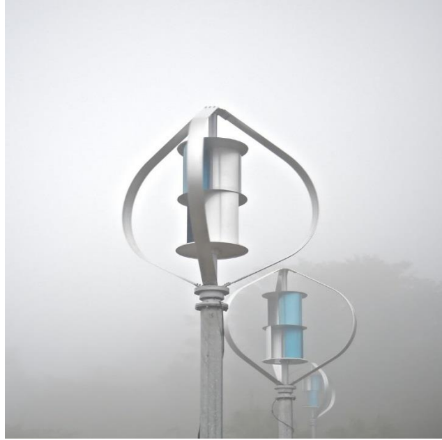
Figure 2-5: Darrieus Wind Turbines With Savonius-Type Start-Up Rotors
