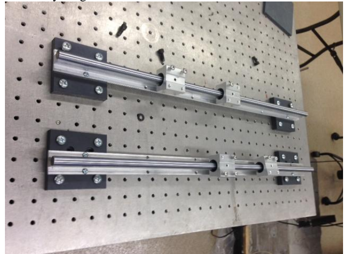
Figure 10: Rail Suspension System
