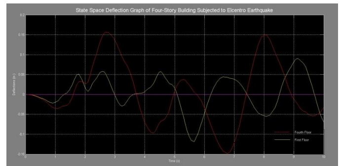
Figure 41: State Space Deflection Graph of Fourth and Second Floor
