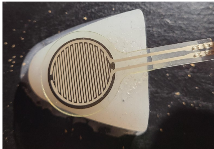
Figure 37: Early Prototype involving Circular Force Sensor for Food Detection
