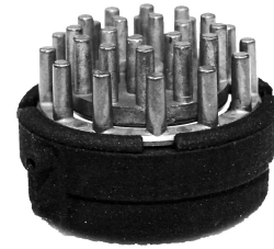
Figure 5: Dry electrode with prongs for separating hair. Taken from the DSI-24 [1]
