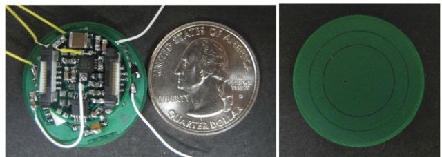
Figure 6: Capacitive electrode for EEG-ECG sensing proposed by Sullivan et. al [58]
