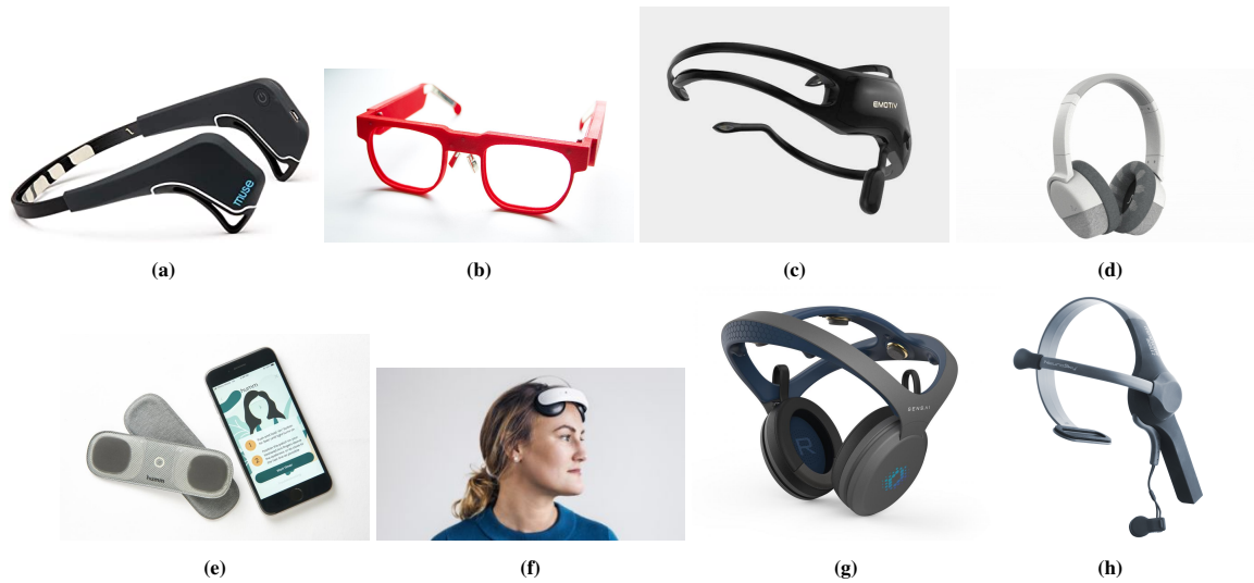
Figure 9: Device appearance for (a) Muse Headset, (b) AttentivU Glasses, (c) Emotiv Insight Headset, (d) Neuroable Headphones, (e) Humm Patch, (f) Flow Headset, (g) Sens.ai Headphones, and (h) Neurosky MindWave Mobile 2
