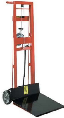
Figure 3. Platform Lift, able to lift 750 lb through a fixed pulley system with crankshaft [11].
