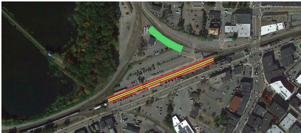
Figure 5.2. Potential Existing Four-Track Station Layout. The yellow lines represent the existing tracks while the red lines represent potential additional tracks. The green rectangle represents the secondary station for the potential Framingham State spur.
