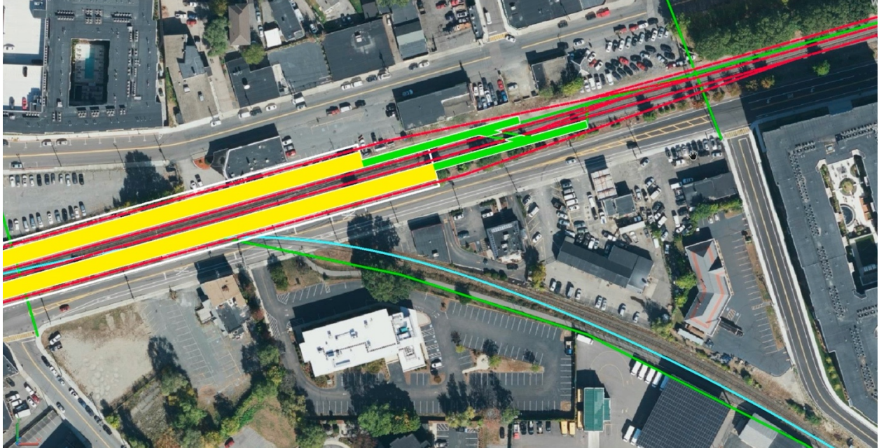
Figure 5.15. Grade-Separated Track Layout on East Side of Station. Green lines show paths, red lines show tracks. The thick green paths are elevated ramps from the ground to the station. The green line to the bottom-right corner goes southeast to the MWRTA bus hub. The green line in the top-right corner connects Marble and Grant street with a pedestrian walkway.
