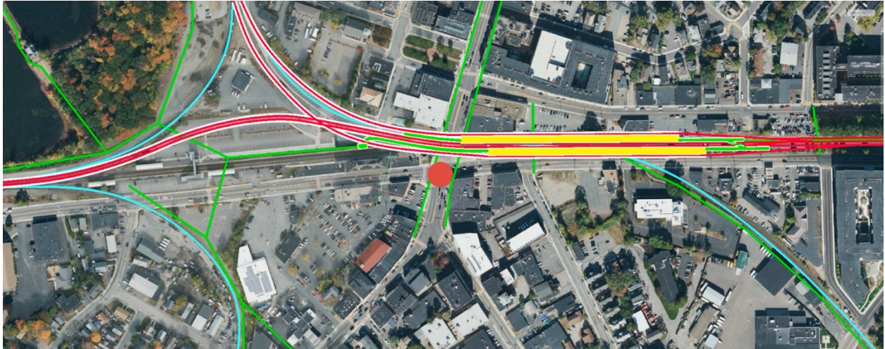
Figure 5.9: Design Plans of Station and Grade Separation. Green shows paths (thicker if above-grade), yellow indicates platforms, red indicates passenger tracks, and cyan indicates freight tracks.
