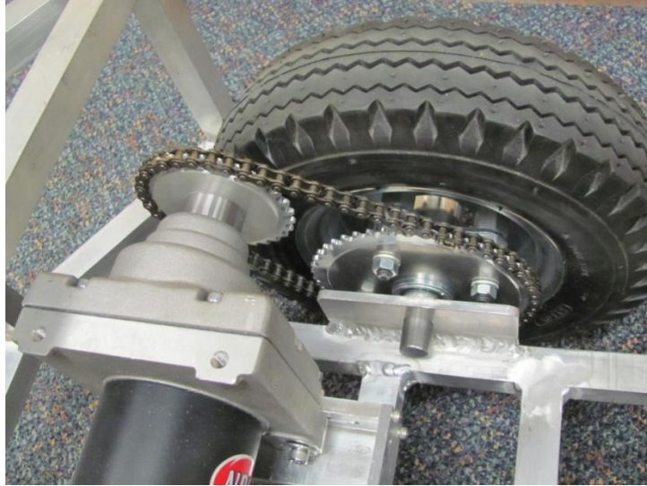
Figure 32: Sprocket and chain completed
