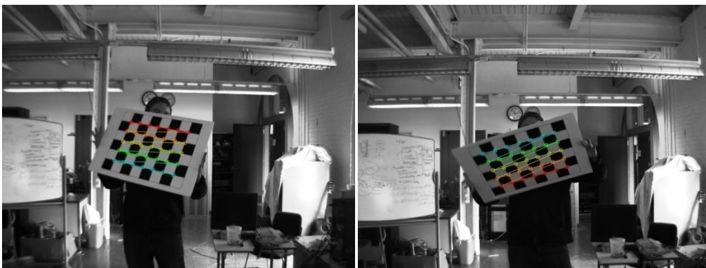
Figure 32: Left image shows chessboard squares recognized in the correct order (top to bottom). The right image shows the incorrect order (bottom-top).
