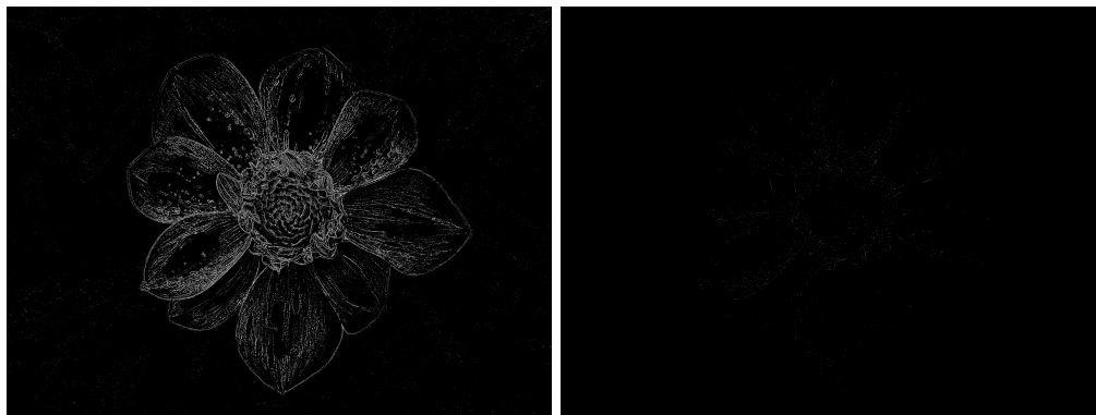
Figure 6: An image of a flower before and after applying erosion with a 3x3 square kernel. The image on the left is the original image. The image on the right has been eroded.
