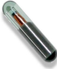
Figure 22 The Megamos Crypto transponder chip picks up the key fob signal and decodes it [54].
