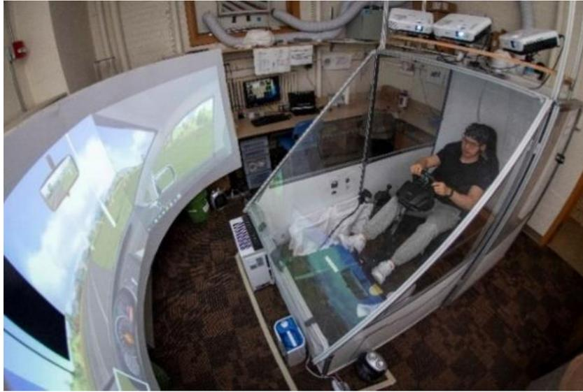
Figure 2. Panorama of the driving simulator cabin ( $\sim 2.94 \text{ m}^3$ ) and screen; The cabin was made of a metal frame, polyethylene boards, and clear acrylic plexiglass plastic boards. The seat was adjusted to make the participant's line of sight fall on the focal point on the apparent horizon line in the in-car environment displayed on this monitor
