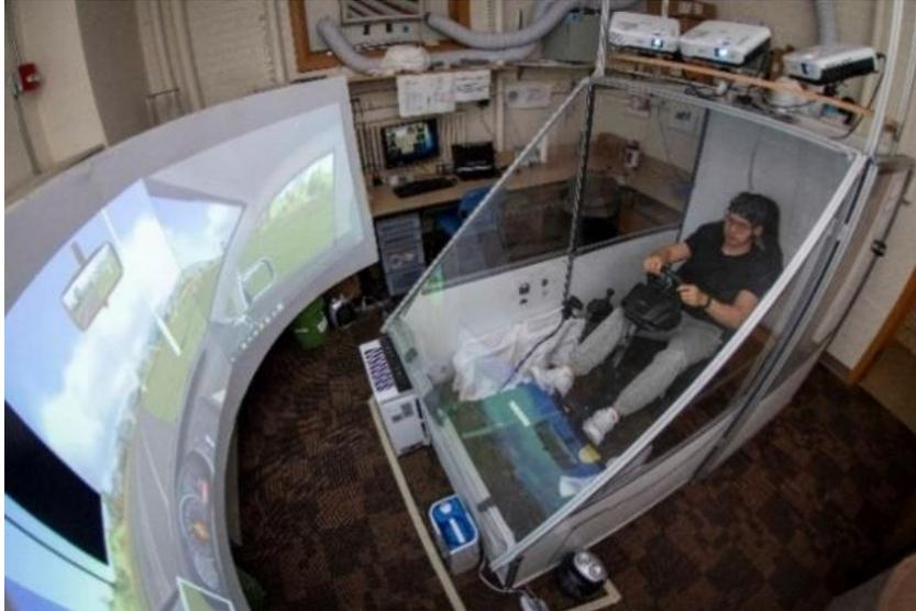
Fig. 1. Panorama of the driving simulator cabin ( $\sim 2.94 \text{ m}^3$ ) and screen; The cabin was made of a metal frame, polyethylene boards, and clear acrylic plexiglass plastic boards. The seat was adjusted to make the participant's line of sight fall on the focal point on the apparent horizon line in the in-car environment displayed on this monitor.
