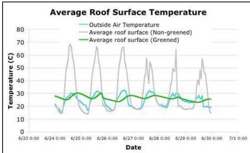
**Figure 2: Rooftop Temperature Comparison (“Center for Green”, 2005)**
