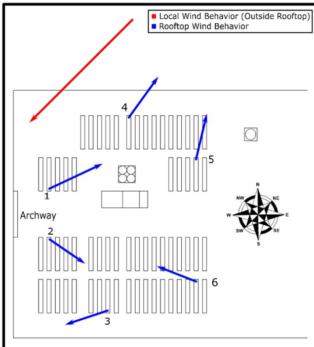
unpredictable. To the left is a diagram showing the wind speeds and directions measured on the farm. Wind speed is indicated by the arrow lengths. From this, we learned that the wind barriers would have to protect crops from all angles. Interviews with other urban rooftop farmers revealed that another farm in Toronto has experienced wind damage to their tomato plants in the past. This showed that the wind problem at
