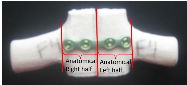
Figure 33: Schematic of how plate centering was measured during pre-testing
