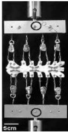
Figure 15: Tethering Gripping System Made of Pulleys and Pivots (Pai et al., 2005)
