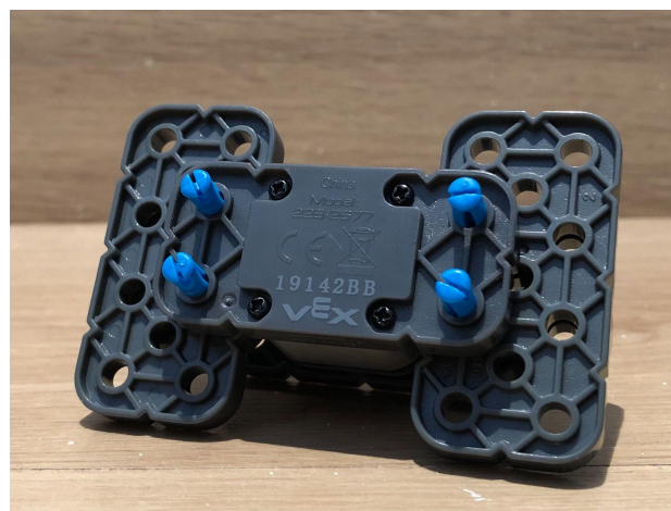
The back of the detached bumper sensor assembly
